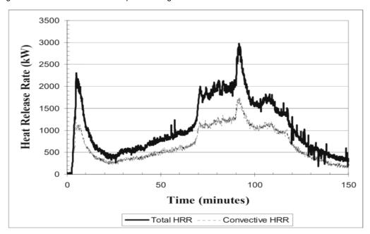
Figure 36: HRR of a front loader tyre – SP Technical Research Institute of Sweden
