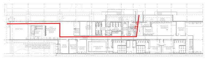
Figure 13: The extended travel distance between alternative exits on Ground floor.
