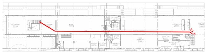
Figure 14: The extended travel distance between alternative exits on Level 1.
