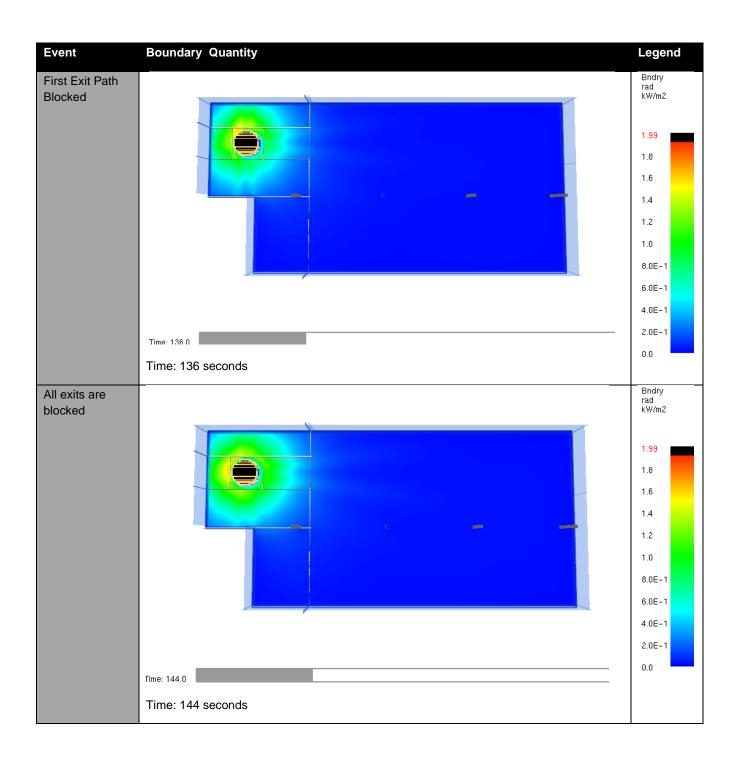
Table 39: Receiving Radiant Heat Flux (Steady State)
