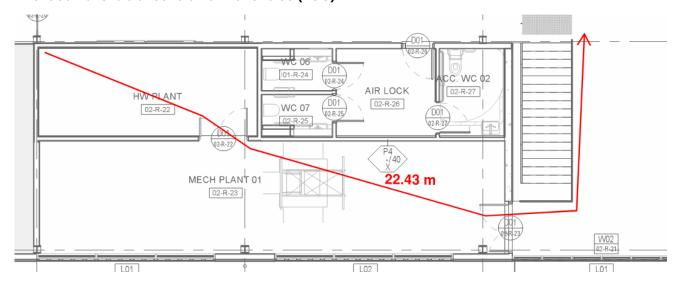
Figure 15: The extended travel distance from Level 1 plant room to a point of choice.
