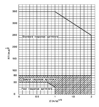
Figure 39: Standard Orientation Sprinkler RTI and C Limits
