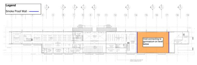
Figure 6: Smoke proof construction on Level 1
