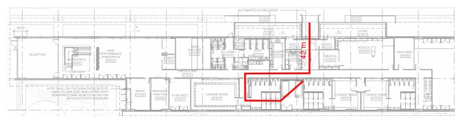
Figure 12: The extended travel distance to an exit on the Ground floor.
