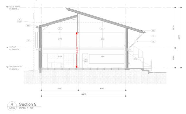
Figure 33: Section view of double height Gym space
