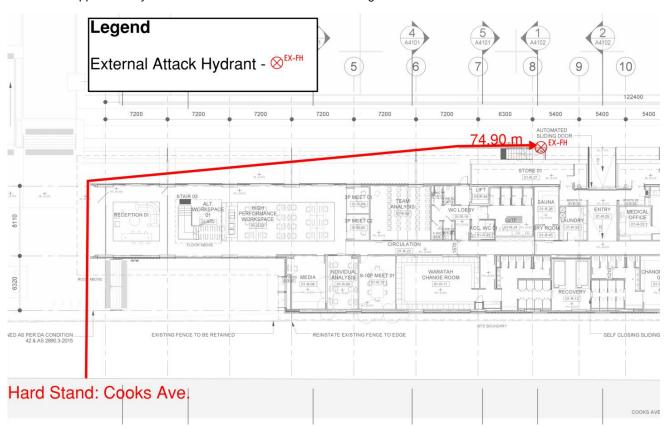
Figure 10: Central external attack hydrant location
