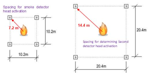
Figure 40: Standard Smoke Detector Spacing (AS, 1670.1, 2015)
