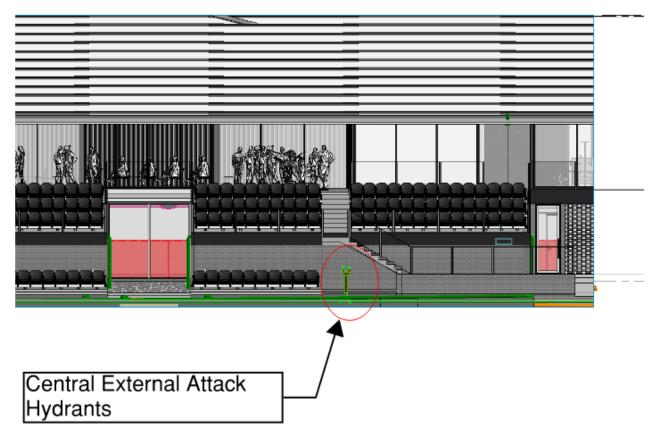
Figure 21: External attack hydrant requiring protection
