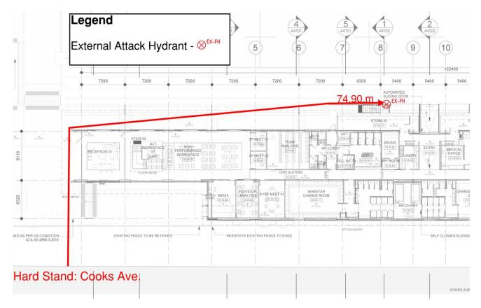
Figure 19: Fire hydrant not within 50 m of hardstand
