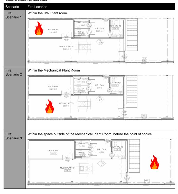
The three fire scenarios consider fire locations that could lead to untenable egress conditions for occupants evacuating from the HW Plant Room. The scenarios presented utilise smoke detectors connected to a Building Occupant Warning System (BOWS) to provide an audible alarm.
